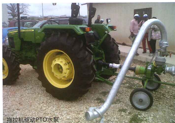
拖拉机驱动PTO水泵
